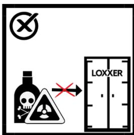
The Loxxer cabinet is not intended for use other than storing and charging Lithium-Ion batteries. For safety reasons, no modifications may be made to the Loxxer cabinet. The intended use is based on compliance with all information in these operating instructions.
